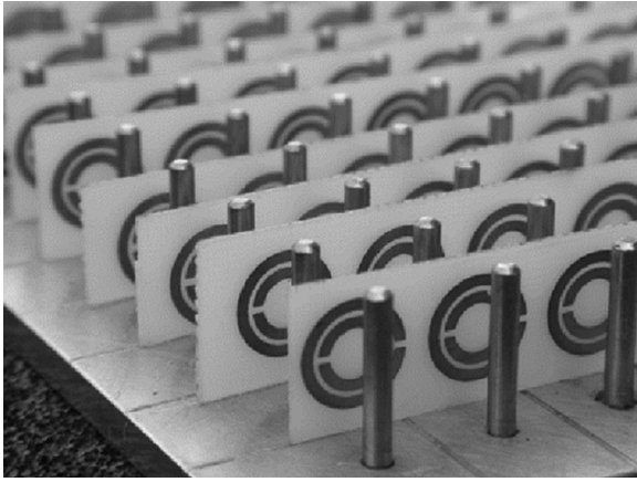
Fig. 4. Combination of structures with a negative permittivity and a negative permeability (experimental implementation).
